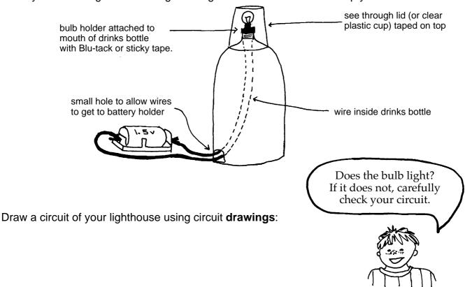
Modify your model lighthouse to make the bulb flash on and off like a real lighthouse. Which component will you need to add?
