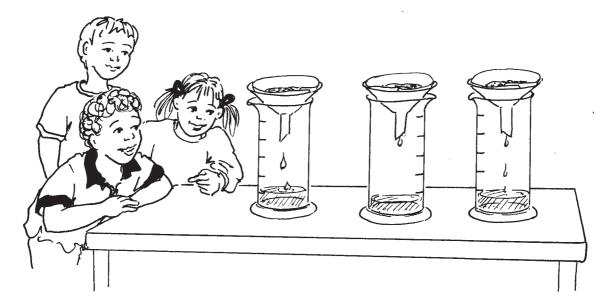
Pour an equal amount of water through each of the samples and measure the amount of water which drains into the measuring cylinders.
